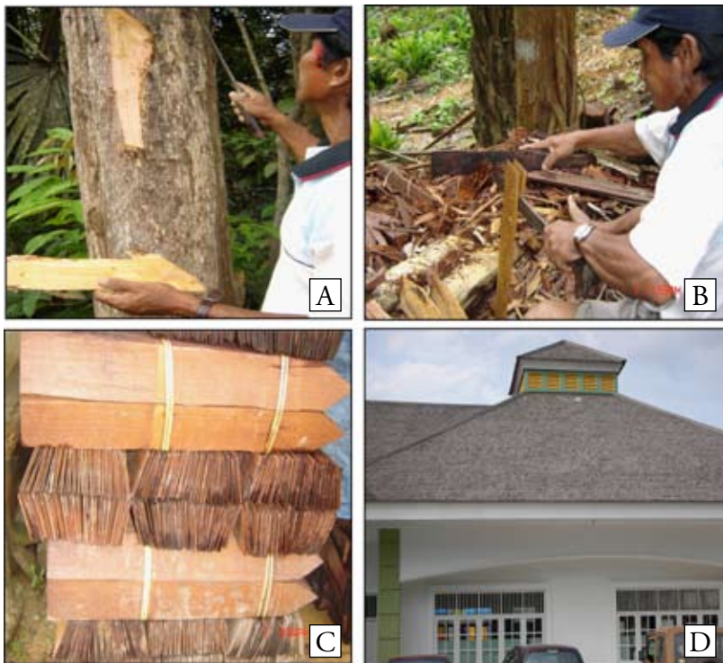
Figure 6.6. Checking the fibre direction; (B) Sirap making; (C) Sirap packets (D) A building with sirap roof.
