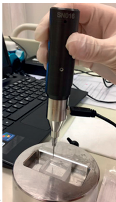
Figure 4: (A) Method of Use of the OsteoProbe® on the midshaft of the tibia after the application of a local anesthetic, (B) measurement performed on the polymethylmethacrylate (PMMA) reference phantom.
