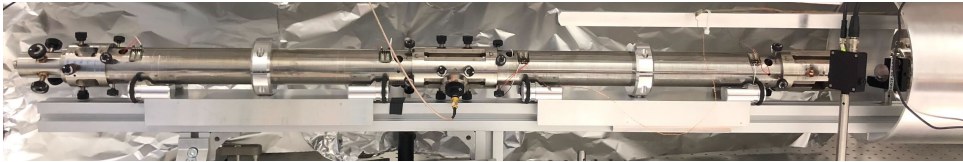
Figure 3.8: Photograph of the filter-cavity mount, showing the first two cavities and the inter-cavity spacer.
