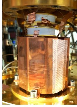
(b) Shield of the four SNSPDs
