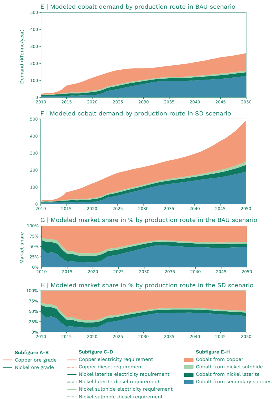
Figure 4.3 - A-B V1 ore grade in the ‘Business as Usual’ (BAU) scenario (A) and ‘Sustainable development’ (SD) scenario (B). C-D Electricity and diesel requirement for each source of metal for the BAU (C) and SD (D) scenarios. E-H Market shares of primary and secondary sources of cobalt for the BAU (E and G) and SD (F and H) scenarios. Note that the y axis in A-D does not start at 0. The data for this figure is available on a repository (van der Meide et al., 2021).
