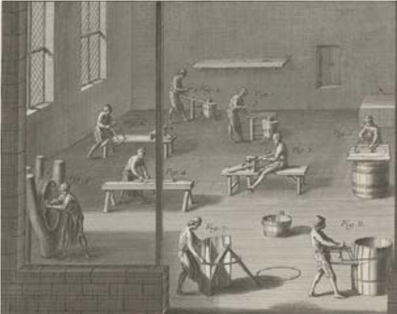
Figure 4.5: The assembly of casks in an 18th-century French cooperage. Figs. 1-3: Reducing and shaping the staves, Fig. 4: Jointing; Figs. 5-6: Assembling the heads, Figs. 7-8: Raising the cask. Fig. 9: Cutting the croze (Fougeroux de Bondaroy, 1777; Plate V).
