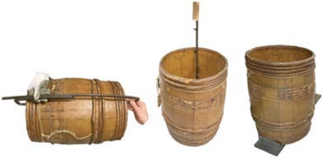
Figure 5.5: Left: Gauge caliper, middle: croze gauge, right: gauge plank (left: Schuif el for herring cask [inv. no. KA 9532], 1722. Amsterdam Museum, Amsterdam, The Netherlands; middle: Kroos el for herring cask [inv. no. KA 9533], 1722. Amsterdam Museum, Amsterdam, The Netherlands; right: Measuring plank for herring cask [inv. no. KA 9972], Unknown date. Amsterdam Museum, Amsterdam, The Netherlands; The casks used in all of the three examples: Half herring cask [inv. no. KA 9921], unknown date. Amsterdam Museum, Amsterdam, The Netherlands).
