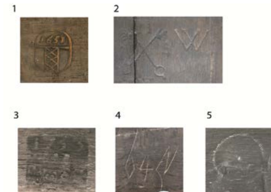
Figure 7.18: Examples of cask gauge marks: 1. Cask gauge approval mark with coat of arms of the city of Amsterdam and the year 1651; 2. Cask gauge approval mark with a simplified version of the coat of arms of Leiden with a "W"; 3. Cask gauge approval mark with the year 1755; 4. Cask gauge approval mark consisting of the numbers 6 and 4; 5. Cask gauge rejection mark consisting of one circle. Sources: 1. Database DANS Data Station Archaeology, n.d., https://archaeology.datastations.nl/dataset.xhtml?persistentId=doi:10.17026/DANS-XQ9-MGH2 , licensed by CC BY 4.0; 2. Verduin, 2019, 255. ID417; 3. Unpublished. ID948; 4. Van der Laan, 2023, 54. ID848; 5. Oosterbaan & Griffioen, 2015, 571. ID573.
