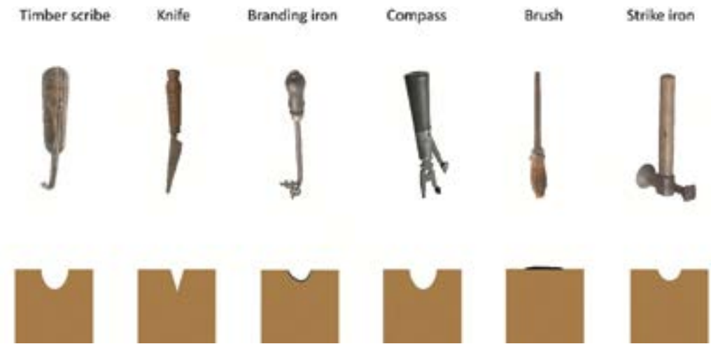
Figure 7.3: An overview of methods of cask mark application: Tools used and a schematic representation of their cross-sectional shapes. Sources: Timber scribe: Scribe for rejection during the gauging of casks [Tool, inv. no. 5708], unknown date. Museum de Lakenhal, Leiden, The Netherlands; Knife: Knife and fork with wooden handle [Tool, inv. no. 4280], unknown date. Museum de Lakenhal, Leiden, The Netherlands; Branding iron: Brand VOC [Branding iron, no. NG-1987-14-1], Rijksmuseum, Amsterdam, The Netherlands; Compass: Scribe and compass [Compass, no. 357.087], Collectie Looij, Nieuwenhoorn. Fotocollectie Rijksdienst van Cultureel Erfgoed, Amersfoort, The Netherlands, reproduced under CC BYSA 3.0. Brush: Brush [Tool, inv. no. NH49-141]. Unknown date. Museum Batavialand, Lelystad, The Netherlands, reproduced under CC BYSA 3.0; Strike iron: Strik iron with number 43 [Tool, no. NG-2013-22-5], Rijksmuseum, Amsterdam, The Netherlands.
