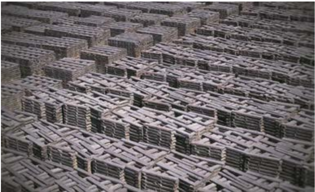
Figure 2.3: Coopers' timber being dried at the present day Vicard cooperage in Cognac, France (Pineau J.L. (2020). Groupe Vicard. Élever la tradition innovation & performance . Retrieved June 17, 2024, from https://www.groupe-vicard.com/files/fr/1591368313.1353/FR_Ctlg_TonnellerieVicard2020-planche.pdf ).
