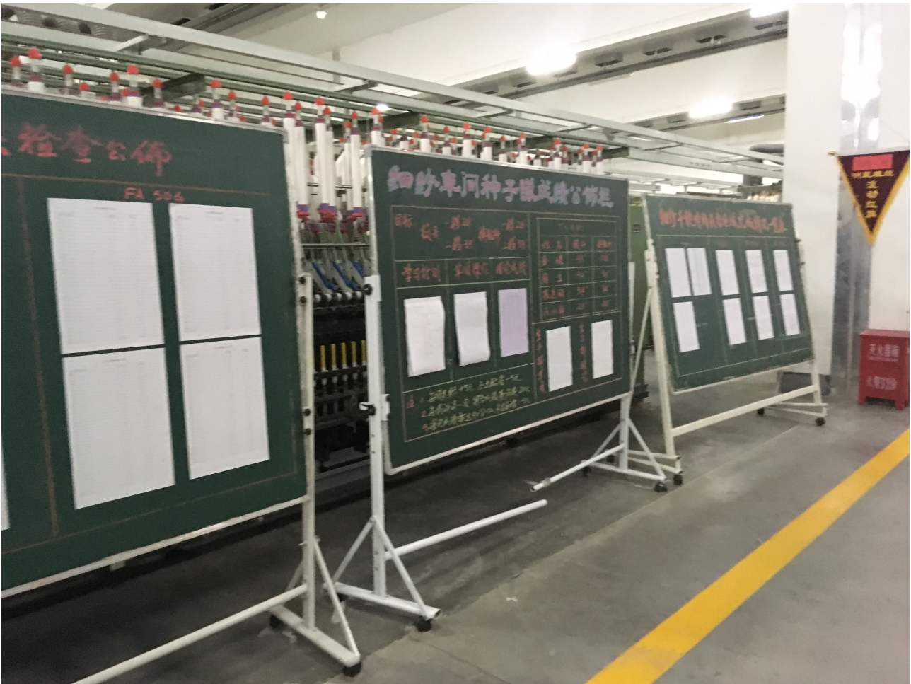
Figure 3.4: The blackboards on shop floors show the results of different levels of inspections in the new factory. The old factory had more blackboards showing individual results of everyday work. Photo taken by the author.
