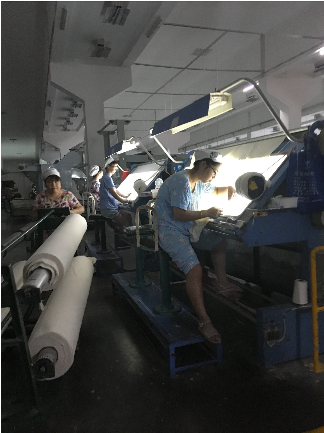
Figure 3.3: The inspectors are finding defects in the cloth in the finishing room of the new factory. They are working under the special light. The finishing room in the old factory and the new factory does not have much difference. Photo taken by the author.
