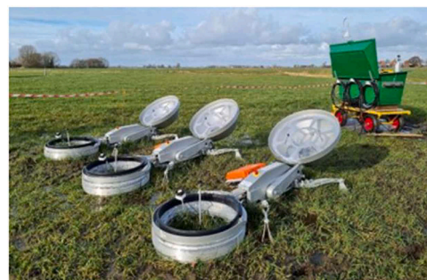
Fig. 1. Setup of the three automatic flux chambers with manual control boards (orange cases) attached onto the side of each chamber. At the moment of measuring, a chamber closes from the ground up after which the lid is placed on top. A small fan maintains a homogeneous trapped air column while heated FEP gas tubes collect and return air samples to the sensor and back. The equipment housing (green cart) containing the ABB-LGR Ultraportable Ammonia Analyzer and other peripherals were positioned behind the chambers (i.e. not in line with the dairy cow stable and the chambers).
