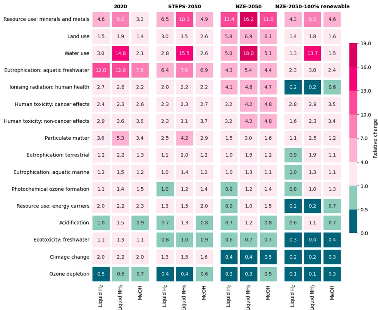
Fig. 5. Environmental tradeoffs of H 2 -based ships in different scenarios from 2020 to 2050 in the S-A-N (11,000 nm-20 knots-Nonstop) scenario. The value represents the ratio of the environmental impact of H 2 -based ships to that of the HFO ship. Note the nature of the scale: impact reductions are values in between 0 and 1, while impact increases are values from >1 to infinity.
