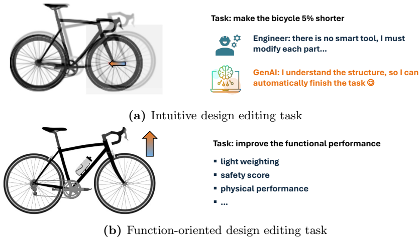
Figure 2.15: Scenarios of engineering day-to-day operation tasks. Inspired by the geometric operation task shown in (a), we assume that with the same optimization pipeline DGMs can also edit the design to achieve a better functional performance.
