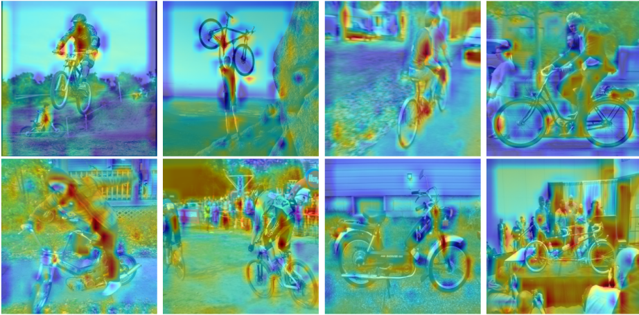
Figure 3.15: Heatmaps of our DAE model on ImageNet images from the bike class. Inception-V3 focuses on the object from the top-classes, such as the bike, and hereby ignores the rest parts of the image, which is suboptimal for evaluating the image plausibility.
