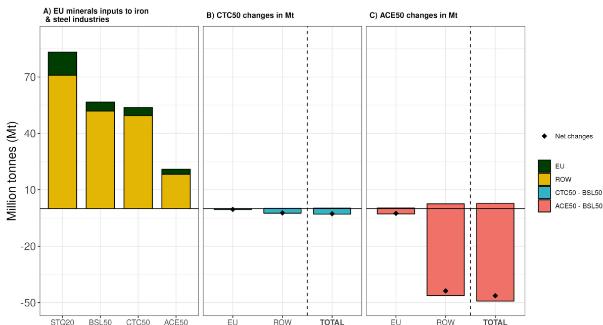
Figure 27. Strategic minerals and iron ore requirements of the EU steel industry and changes in requirements for the CTC50 and the ACE50 scenarios compared to the BSL50 scenario
