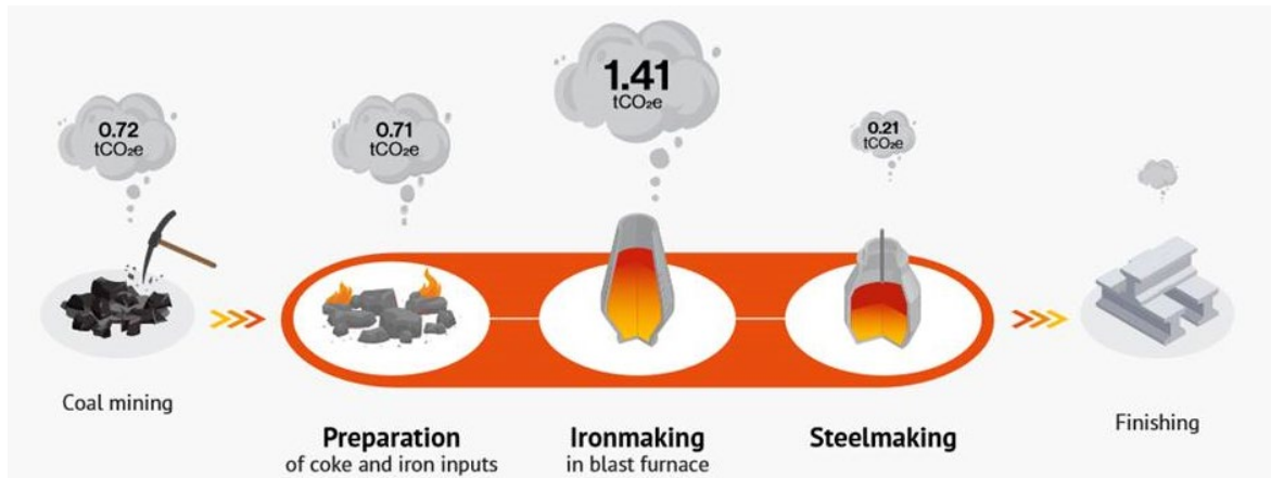
Figure 1. Overview of the main hotspots for GHG emissions in iron and steel making production via blast furnace and blast oxygen furnace route
