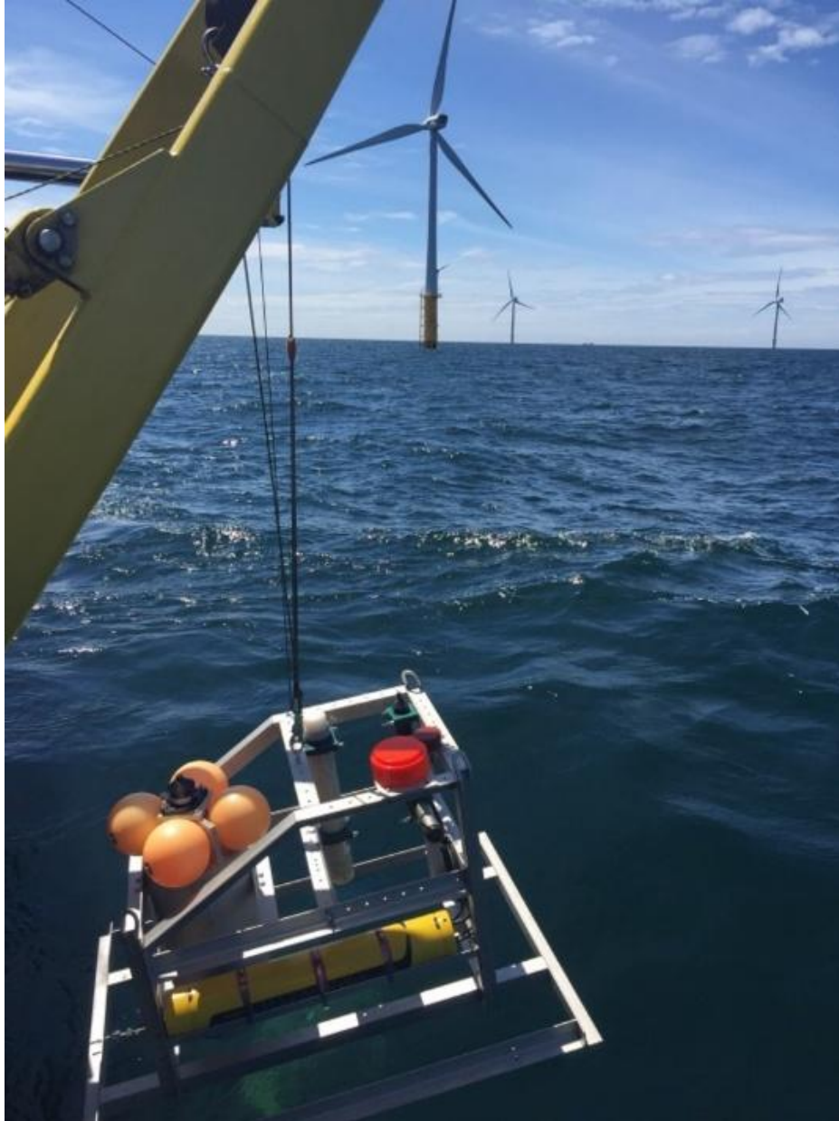
Figure 5: Picture during deployment of monitoring sensors for a study as part of this thesis. This frame was designed by LifeWatch and the Flanders Marine Institute (VLIZ) and allowed for multiple sensors to be deployed at once. The yellow cylinder mounted horizontally is an echosounder that allows tracking of free-ranging fish. The grey cylinder mounted vertically is a C-POD that records the vocalisations made by harbour porpoise ( Phocoena phocoena ). This fieldwork picture was taken from the Belgian research vessel Simon Stevin.
