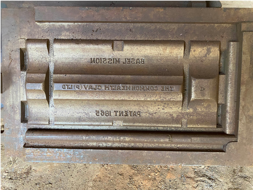
Figure 10.17: Metal mould of the tile from the Commonwealth tile factory. Source: Priya Joseph.
