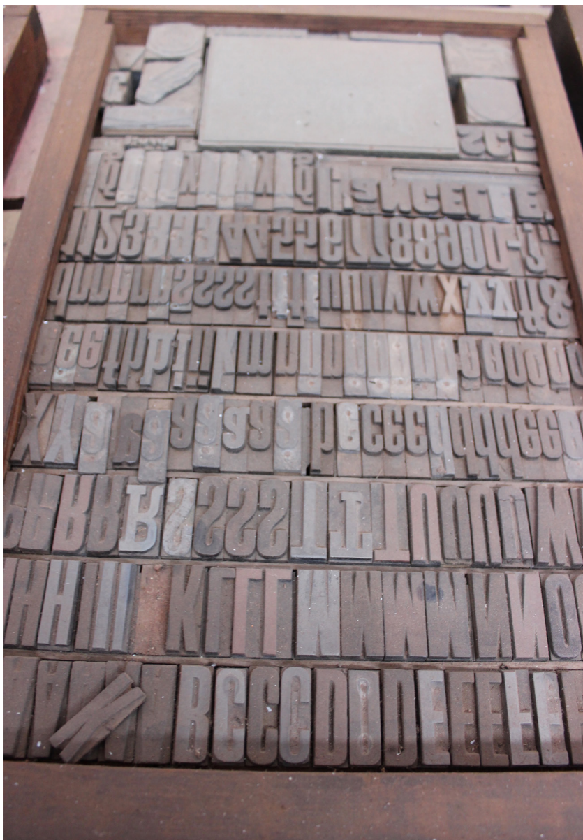
Figure 10.4: Roman print type block for letter pressing, Basel Mission Printing Press, Mangalore. Source: Author. 16
