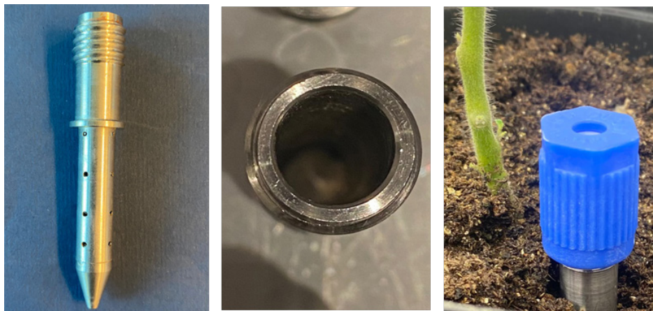
Supplementary Figure S1. Non-invasive set-up to sample root/rhizosphere associated volatilome in planta. Hisorb probes were inserted into cylindrical holders made of stainless steels, and buried for approximately 5 cm deep in the soil near tomato roots to trap root-associated volatiles. The cylindrical holders have small perforated surface preventing soil contact, creating headspace and allowed passive diffusion of volatile compounds toward the probes inside the holders. Screw caps on the holders enabled secure closure to minimize contamination of volatile compounds emitted by aboveground plant tissue or by environmental backgrounds.
