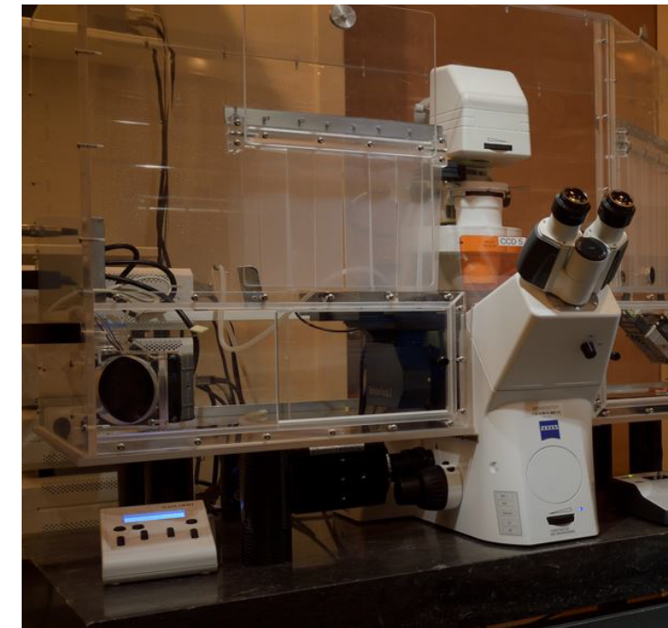
Figure 1: Picture of the microscope, including the climate control chamber surrounding the microscope, maintaining the levels of CO 2 constantly at 5% and temperature at 37°C.
