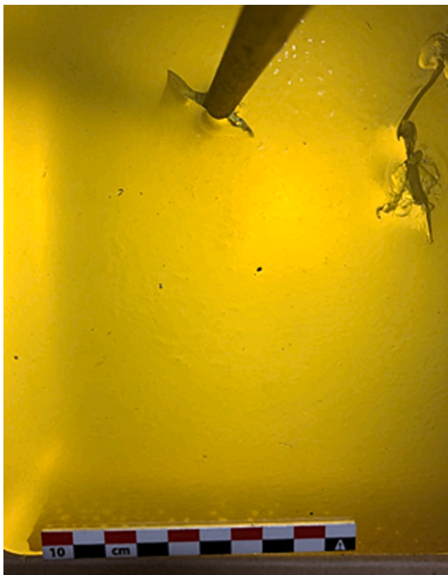
Fig. 5. Photograph of a typical “wound” from an experimental shot. Photo: Mick van Harderwijk.
