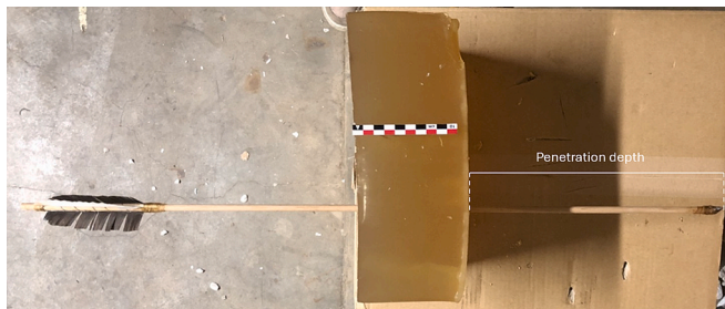
Fig. 4. Photograph of arrow after penetrating the gelatin target indicating the measured penetration depth. Photo: Mick van Harderwijk.
