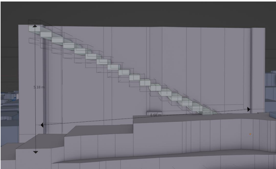
Figure 157. Visualisation of reconstruction range, using different riser and tread dimensions. The lower option has a reduced riser height (18 cm instead of 20 cm). The higher has both an increased riser height (22 cm) and tread length (42 cm).
