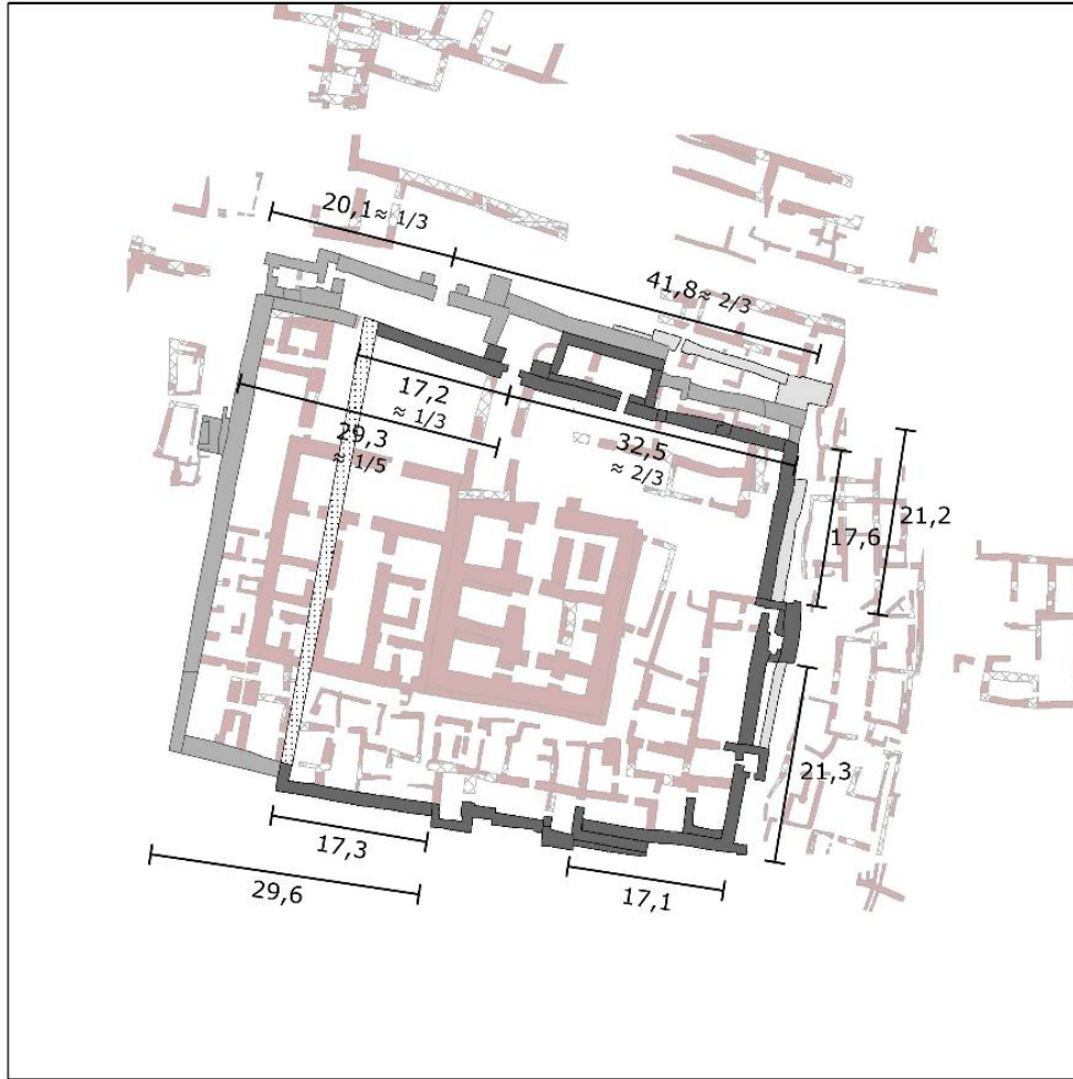
Figure 200. Dimensions of the fortification, indicating regularities with regards to placement of main gate (old and new) and other defensive features.
