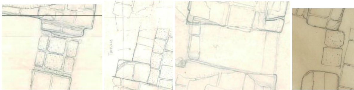
Figure 121. Different threshold constructions in the Dunn. 1: full width of wall, bonded with jambs. An example of a neatly constructed one in the residence. 2: Consisting of two baked tiles with some space between, probably a gutter for drainage of the main court. 3: Bricks on their sides applied on both ends of a doorway, which functioned as small retaining walls for a loam fill in the middle. 4: two bricks without special features.
