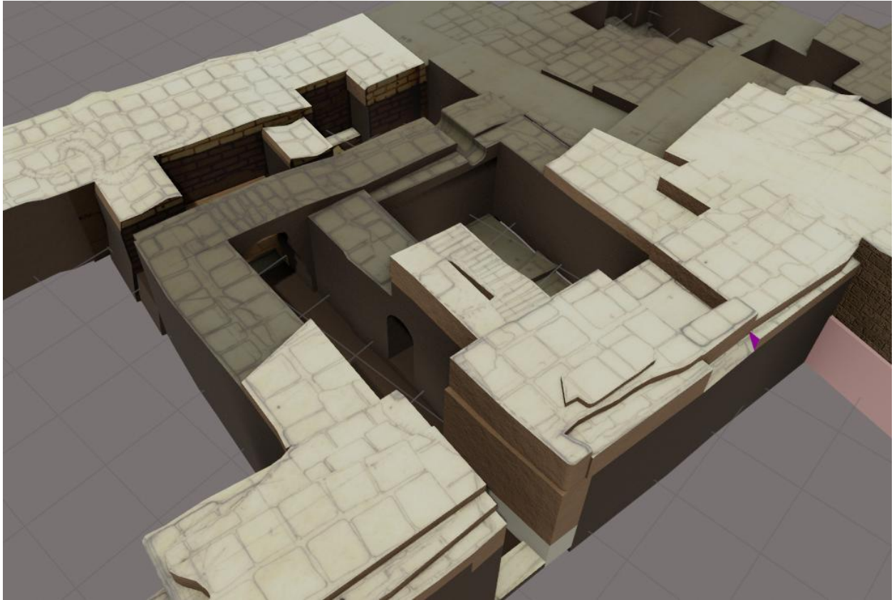
Figure 86. Layered differences in masonry material and structural characteristics, indicative of either a renovation phase, or logistics of construction. North-western corner, building NW-3.
