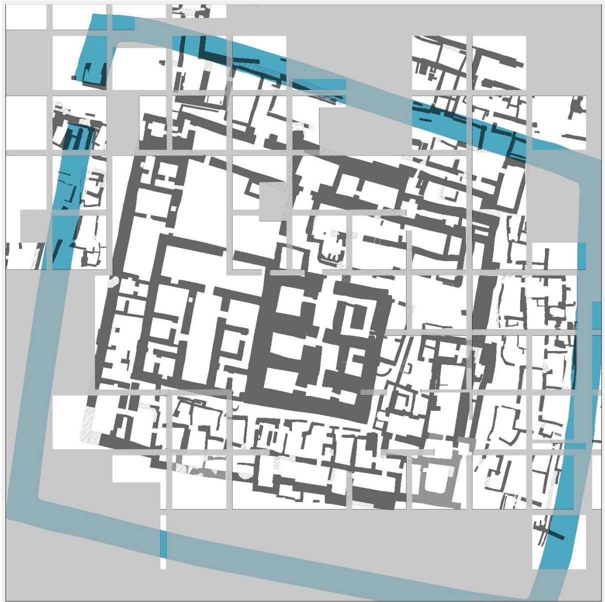
Figure 2. Plan of the Dunnu including all excavated architecture, all phases combined. In blue a fosse surrounding the settlement. Grid blocks are 10x10 meters.
