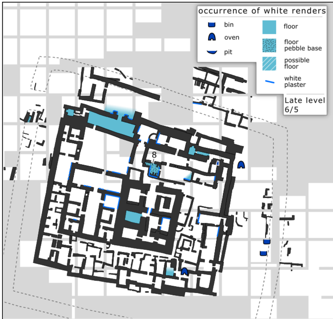
Figure 63. Late level 6/5. Evidence for white renders in the Dunnu. For some areas indicated on the figure, already rendered in early level 6/5, it is uncertain whether the white render was maintained also in late level 6/5.
