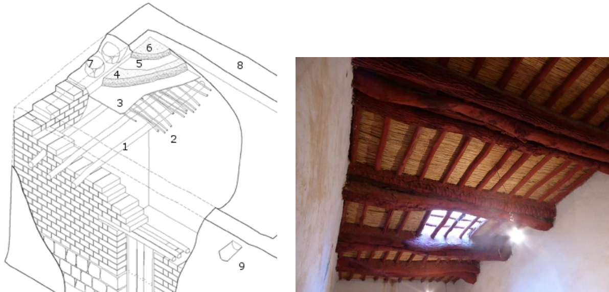
Figure 53. Roof construction methods. Left: common roof construction of houses in northern Syria. 1. Joists of poplar. 2. Purlins of brushwood. 3. Matting. 4-6. Layers of loam mortar with plastic sheet in between. Final layers mixed with dung or very fine clay to increase waterproofing. 7. Stone reinforcement. 8. Low parapet. 9. Water discharge. (after Dipasquale, Onnis and Paglini, 2009, fig. 63). Right: roof construction for a room with a larger span. The joint beams are a combination of trunks of date palm and tamarisk. It is a construction method that can be used when strength is required, but proper timber is not available. Top floor in a fortified building in south-eastern Morocco (photo by author).
