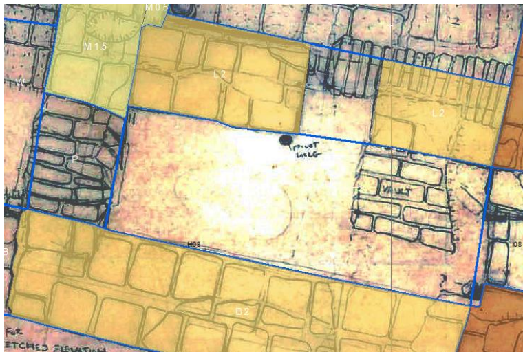
Figure 98. Remains of vault of corridor space NW-3d, "Tammitte's office". On the left the part that covered the doorway, which was lower thus better preserved. It applies wholes and 1/3-size bricks. The row of mud bricks placed on their side in the room directly to the north, may also indicate the pitched brick vaulting technique was used.
