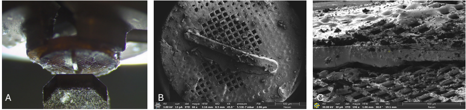
Figure 5.4: Initial trimming attempts of HPF root tissue to reduce sample volume for subsequent milling with a FIB/SEM ion-beam. (A) A HPF radish root tip was successfully attached to a grid using cryo-glue, and trimming was initiated with a diamond trim-knife in a cryo-ultramicrotome. (B) After initial trimming, the sample was transferred to a FIB/SEM (Aquilos, Thermo Scientific TM ) for assessment of vitrification quality and the trimming procedure. (C) During further milling with an ion-beam, significant contamination from redeposited excess material on the milled surface became apparent. Images were created in collaboration with Depelteau (2022) [163] as part of a joint study. These images were first published in Depelteau (2022) [163] and are included here with permission.
