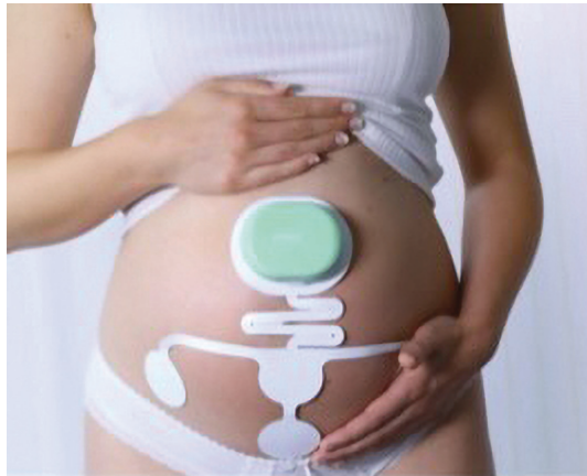
Fig. 1. The NFMS (Nemo® Fetal Monitoring System, Nemo Healthcare B.V., Veldhoven, The Netherlands) consists of a base, a link and a self-adhesive patch incorporating six electrodes.
