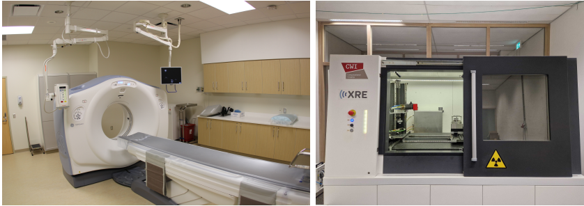
Figure 1.1: Comparison of a medical CT scanner (on the left, photo credit [44]) and a laboratory micro-CT scanner (on the right).
