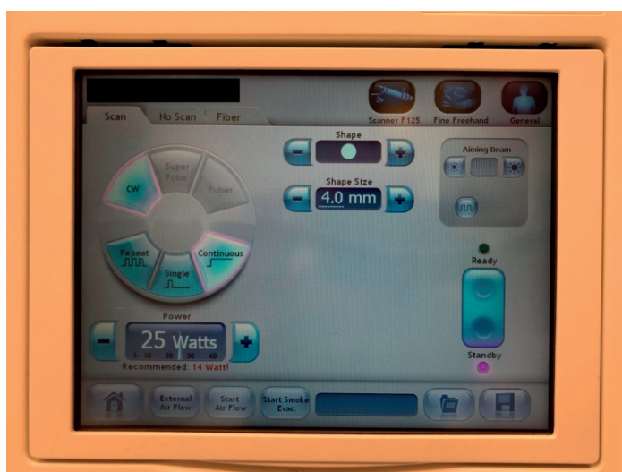
FIGURE 3. PHOTO OF LASER SETTINGS, STANDARD LASER SETTINGS FOR CO 2 LT ON THE LASER SYSTEM USED.
