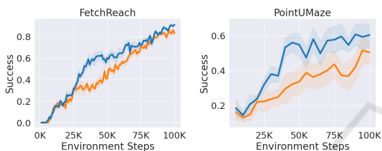
Figure 5: IMGEP with (blue) and without (orange) post-exploration. Left: Performance on FetchReach, with results averaging over 10 different random seeds. Right: Performance on PointUMaze, averaged over 10 different random seeds. Overall, agents with post-exploration outperform agents without post-exploration.
