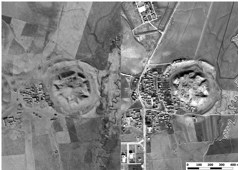
Figure 5.3: State-of-the-art sensors, such as WorldView-2, can resolve the ground in great detail, on the right. CORONA provides historical evidence of land-use land-cover changes, on the left. In this particular example, one can assess the impact of modern buildings on Tell Beydar. Image resolutions are comparable despite the age of spy-satellite imagery.
