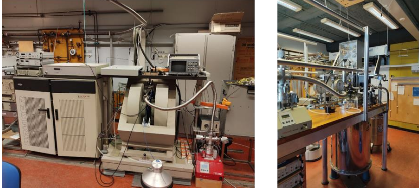
Figure 1. Spectrometer used for electron paramagnetic resonance (EPR). Left: Bruker Elexsys E580 9 GHz EPR spectrometer, operating magnetic field 0-0.5 T. Right: Homebuilt 275 GHz EPR spectrometer, operating magnetic field 0-11 T. Here the magnet is a superconducting coil immersed in liquid helium.
