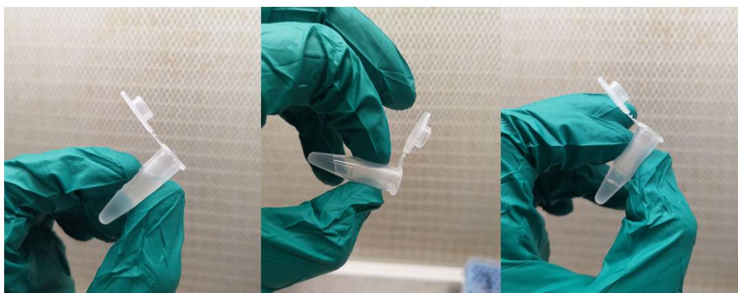
Fig. 5 Washing beads with PBS. Due to the high surface tension more liquid will remain in the 1.5 mL tube. Tip over the tube without excess shaking to avoid losing beads
