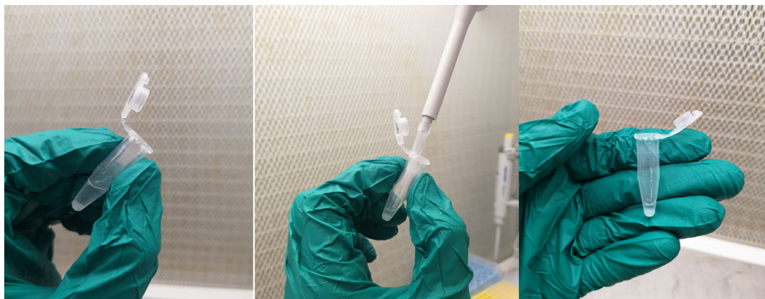
Fig. 6 Taking off the supernatant by pipetting. Make sure to leave a volume equal to the pellet volume to avoid aspirating beads
