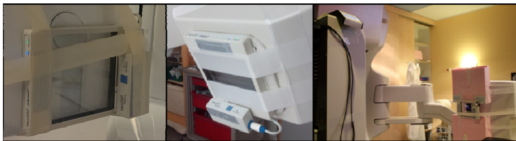
Fig. 3. A kerma-area product meter attached to a dental scanner, a C-arm and a guidance system of a linac (from left to right). To avoid contact between the meter and the tube case of the guidance system it may be necessary to add a polystyrene separation.
