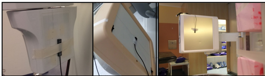
Fig. 4. A solid-state probe attached to the flat panel of a dental CBCT, a C-arm for angiography and a guidance system of a linac (from left to right). The position of the meter must be marked for the sake of reproducibility.
