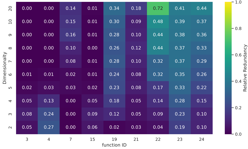
Fig. 3: The average Relative Redundancy Factor over all instances for the CMA-ES using the ‘RESTART’ strategy for the BBOB functions with any redundant restarts. The grid shows the RRF (Eq. 7) per dimension and function individually.
