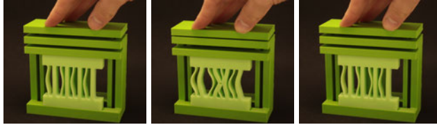
Figure A.2: A hand-operated flexure based device (dark green) containing a smaller n = 4 beam counter illustrates the robustness of our design.
