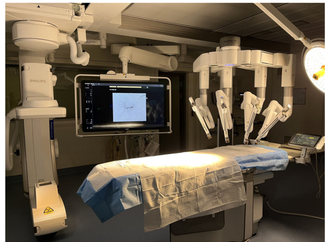
FIGURE 1 Hybrid operating room equipped with cone beam computer tomography and Da Vinci operating robot.
