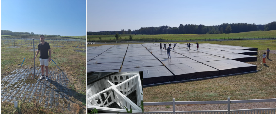
Figure IV: Different LOFAR antennas. On the left, a low-band antenna is shown with a human for scale. In the middle below, an image of a high-band antenna is displayed, which is concealed beneath the tiles on the right, with humans standing on top for scale. These pictures were taken at the PL612 station in Bałdy (Poland) by the author and his colleagues.
