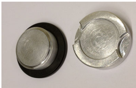
Fig. 4 Metallic plates made to hold and equally distribute heat and pressure when melting the parafilm and finalizing the flow cell
