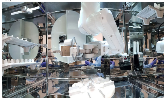
Fig. 2 (a) The outside of the APOTECaChemo robot that is used for robotic compounding. (b) The working area of the robot with the robotic arm, the dosing device and gravimetric control.
