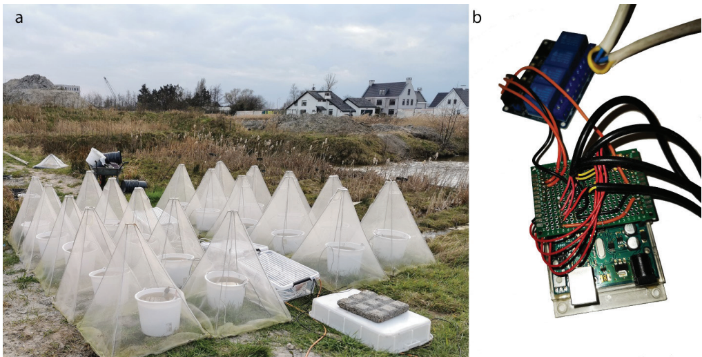
Figure 3.3 Overview of the experimental setup. Panel a shows the mesocosms covered by emergence traps and the HHHI and power strips in the middle. Panel b shows the HHHI, with the Arduino and circuit board to the left, and the relay board to the right.
