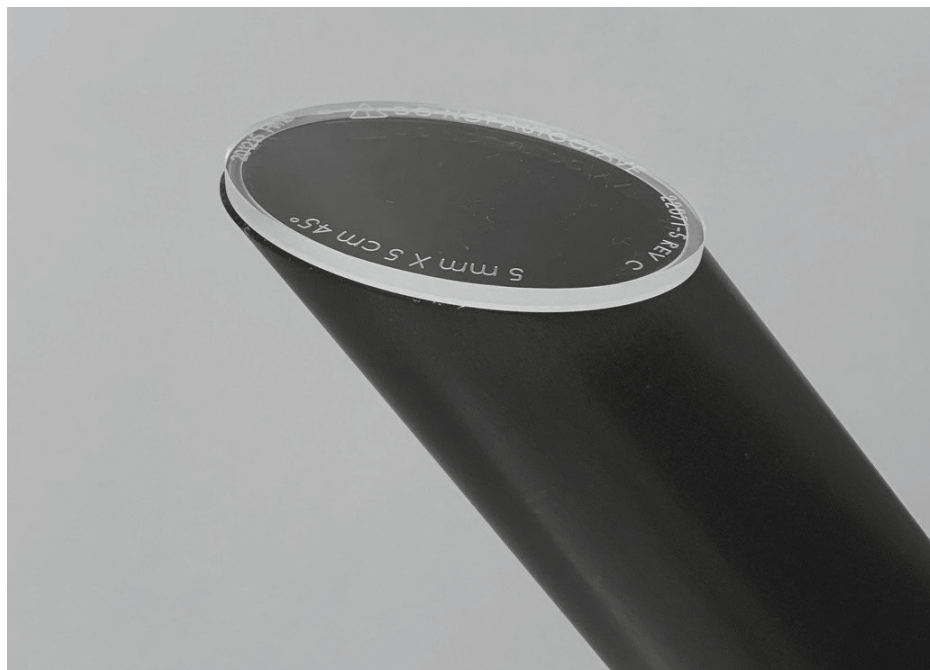
Figure 2. Picture of the tissue-equivalent polymethyl methacrylate (PMMA) bolus attached to the IOERT applicator exit to move the maximum dose to the tissue surface.
