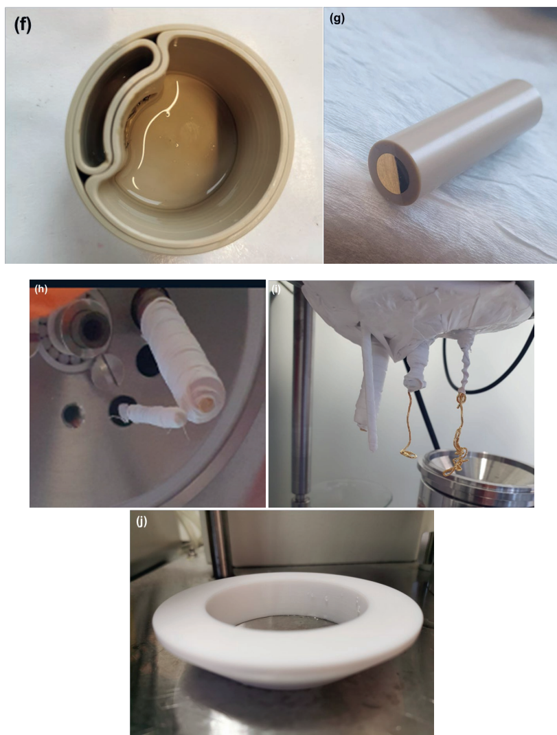
Figure E.1 Several pictures from the high-pressure electrochemical rotating disk electrode cell and its components (a) main mechanical parts of the high-pressure cell; (b) electrochemical parts of the high-pressure cell; (c) PEEK cup and membrane separator, and Teflon cylinder in the stainless steel vessel; (d-f) PEEK cup and membrane separator; (g) rotating disk electrode (gold); (h-i) reference electrode, thermocouple, and all other metal surface covered with Teflon tape; and (j) Teflon cylinder used to decrease headspace.
