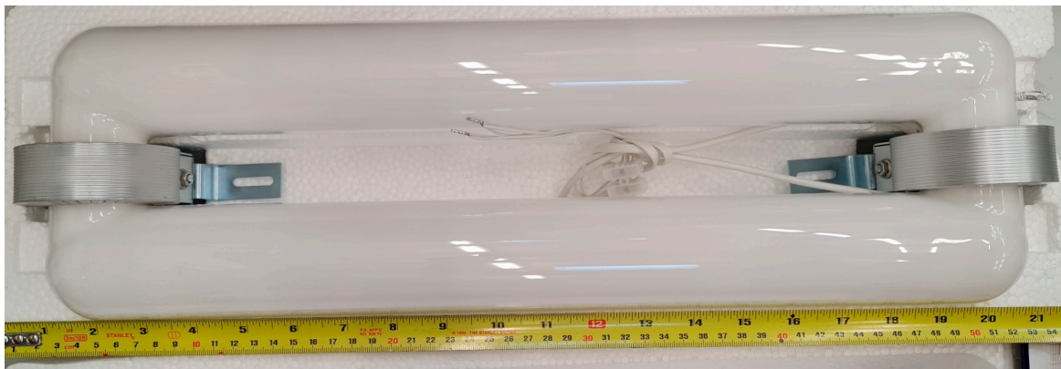
Figure 1. Commercial LTTS-LVD300SB electrodeless fluorescent plasma lamp (i.e., a diameter tube of 56 mm and a total length of 1120 mm) to test its high coupling efficiency.
