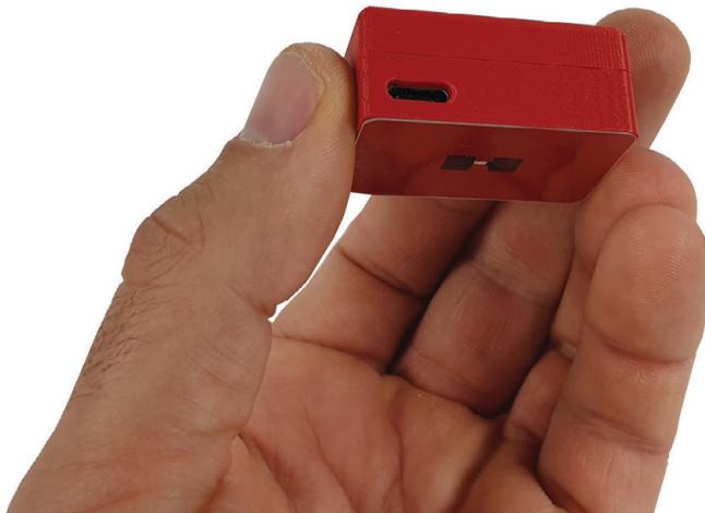
Figure 1. Picture of the penile self-developed sensor (measuring 41 x 27 x 19 mm) The sensor settings are based on the information from the sensor description of the functionality options, set on measuring underneath the skin of the penile shaft [16].
