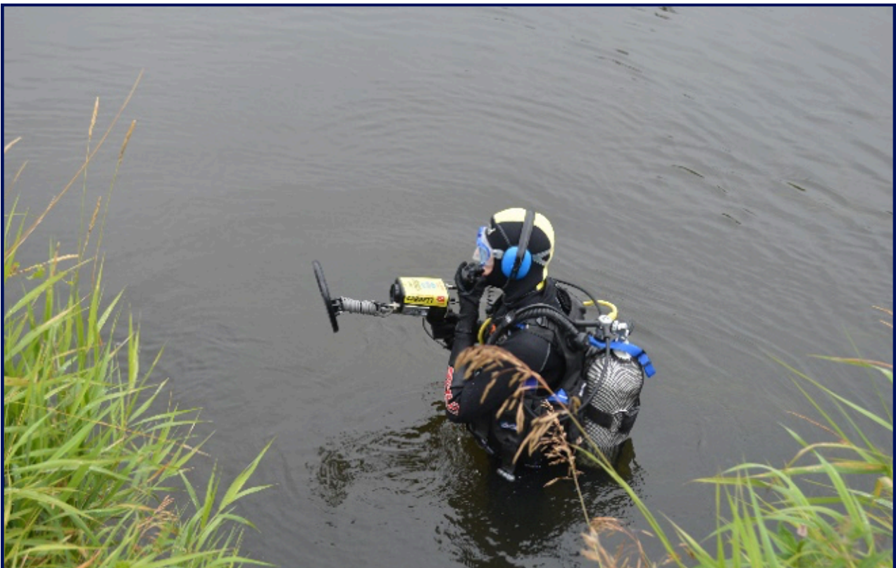
Figure 8: a diver is going to use the metal detector underwater (Project photo).
