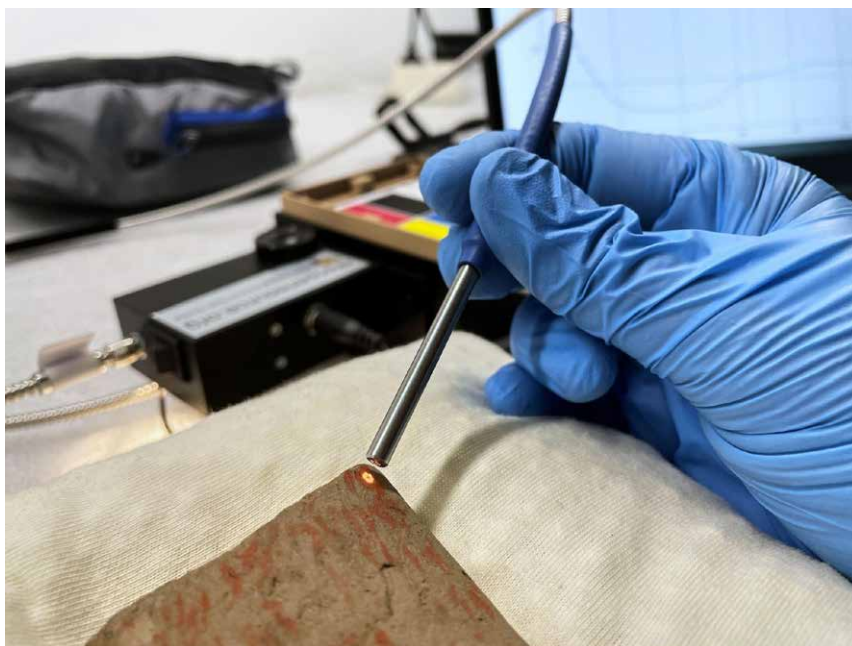
Fig. 4.6: FORS measurements on figurine F 1941/8.6 (red ink and clay medium) (© VIEW – KU Leuven).
