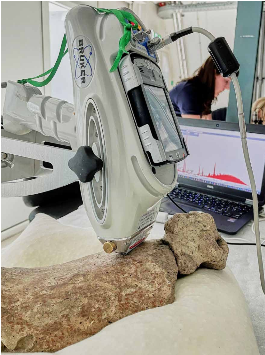
Fig. 4.5: pXRF measurement on figurine F 1941/8.1.
