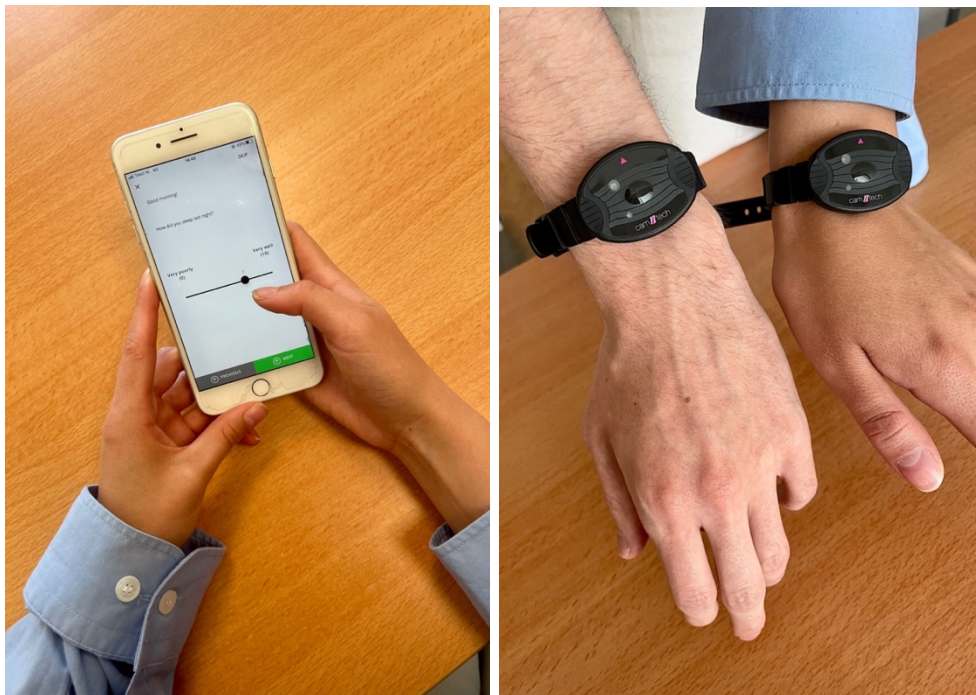
Figure 2. Visualizing the Use of the Ecological Momentary Assessment (EMA) Application (left) and Actigraphy Device (MotionWatch 8 ©) (right)
