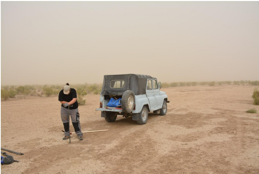
Figure 6.39 The figure shows the coring of the first hand auger core (TGK_Cr_1) at the center of Paleochannel 7 in the Togolok area. The paleochannel is located approximately 600 m from the main mound of Togolok 1.
