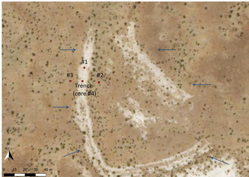
Figure 5.43 The image shows the paleochannel (blue arrows) and the coring points (#) along the cross-section. The middle point indicates the test trench position and core n. 4 at the bottom of the trench.
