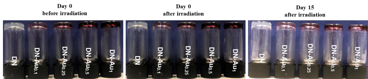
Figure S4. Gel inversion test before and after UV irradiation at Day 0 and at Day 15 at the end of the experiment.
