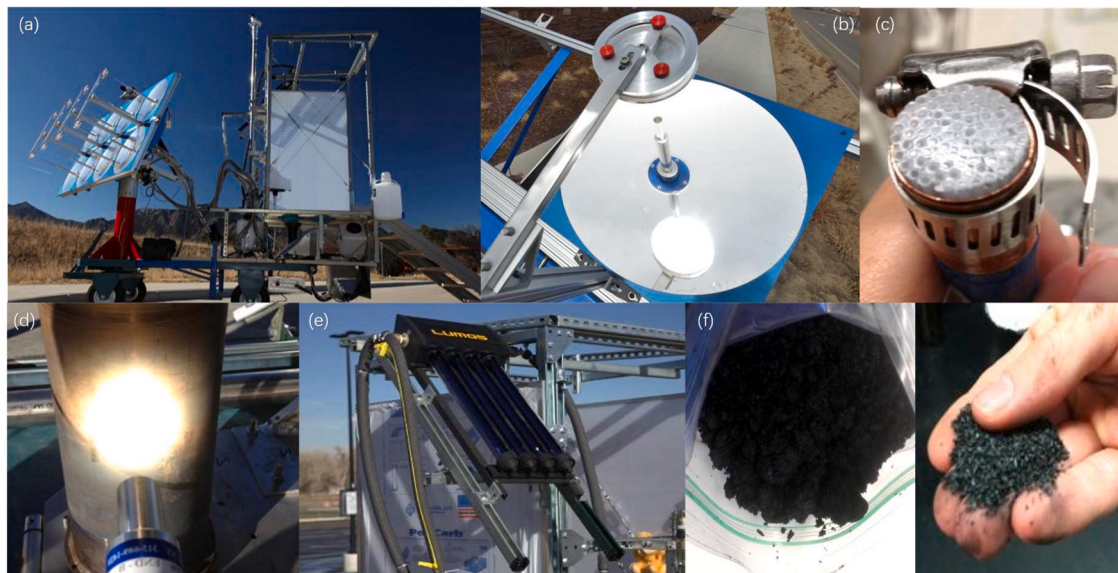
Fig. 1. Sol-Char sanitation system (a) Overview (b) Solar concentration system (c) Optical fiber bundles (d) Pyrolysis reaction tank (e) Solar collector for urine disinfection and (f) the biochar converted from human feces by solar pyrolysis.
